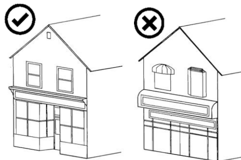
Examples of appropriate and inappropriate alterations to storefronts (Source: Unionville HD Plan)
