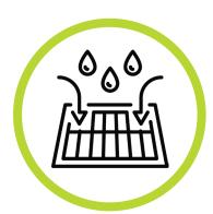
**Catch Basin:** A curbside opening that collects rainwater from streets and serves as an entry point to the storm drain system.
